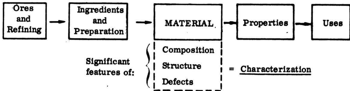
Image 2: This diagram in the Materials Advisory Board’s 1967 report portrays characterization as a critical step on the road to effective use of materials. From Materials Advisory Board, *Characterization of Materials*, 1-9.
