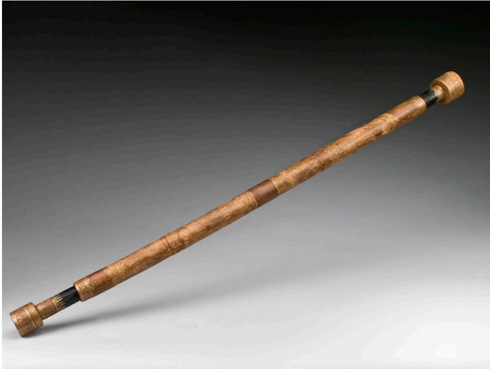
Figure 2: Replica of an early Galilean telescope. Its length is 2 feet, 8 ½ inches. Source: Science Museum Group Collection Online .
